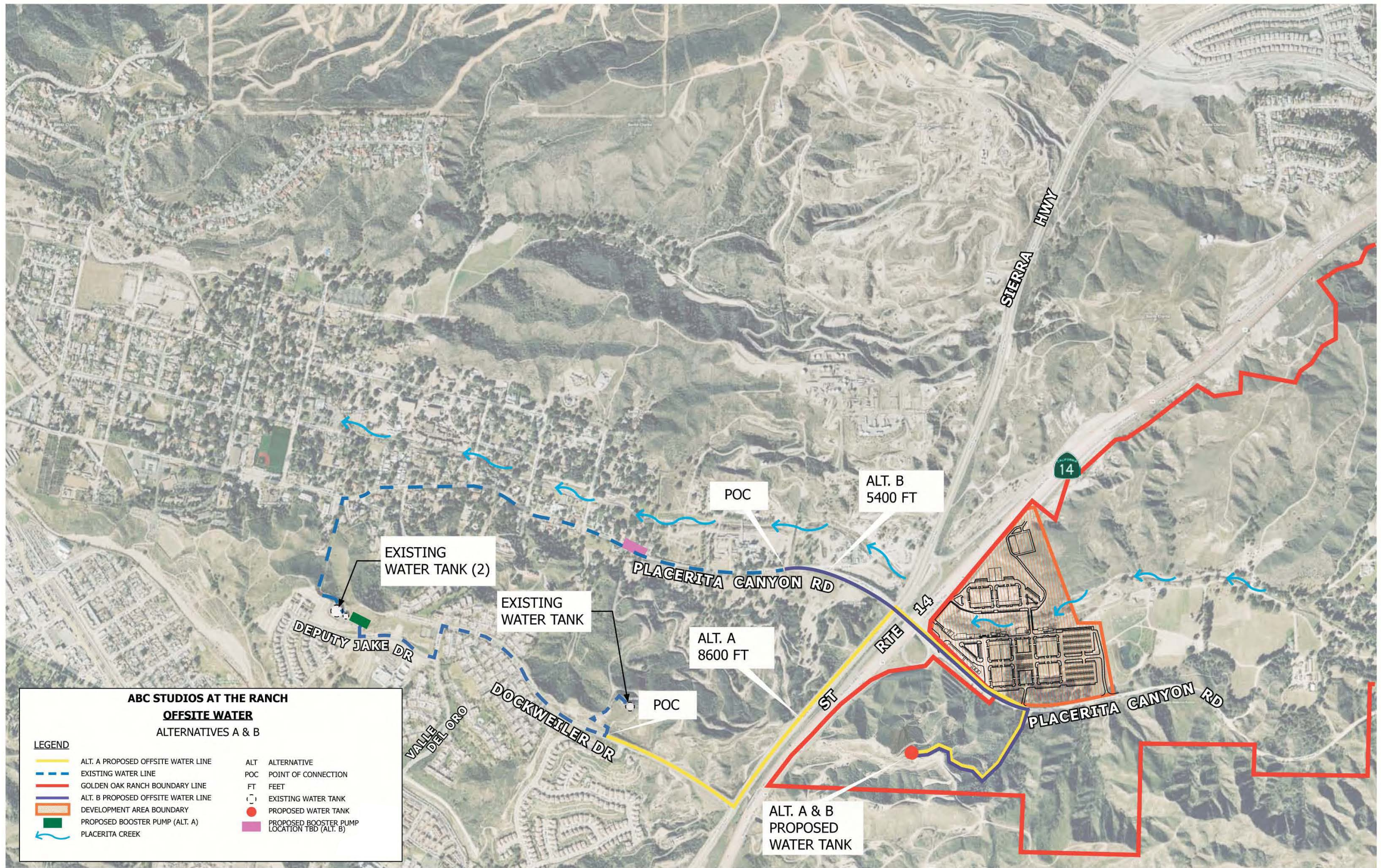
Alternatives A and B Off-Site Water Improvements Disney | ABC Studios at The Ranch
